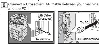
(Right Side of Machine) NOTE: Do not use Standard LAN Cable.
